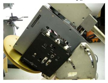
The Paramount has been upgraded with a new control system from Software Bisque. The MKS4000 system uses the same control boards and servo motors as the Paramount ME, so we know it is reliable and thoroughly field tested by hundreds or thousands of users. Our friends Steve and Tom Bisque have been very generous in their support of ATMoB in the past, and that generosity has been magnified a hundredfold with an 80% discount on the MKS4000. Please mention your gratitude to them whenever possible
